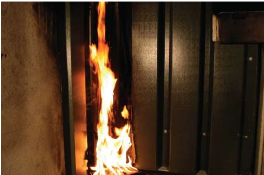
Figure 7. Reaction to fire: single burning item test
