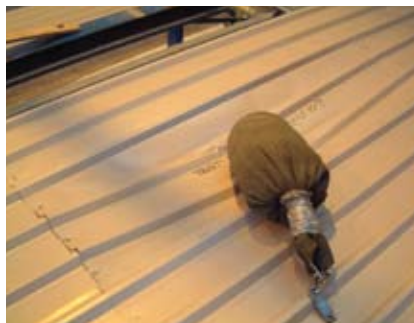
Figure 6. Successful non-fragility test with minimal damage on nominal 0.7 mm gauge liner
