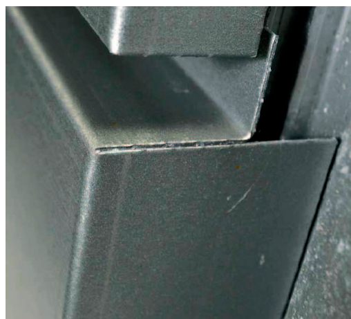
Detailed view of the cut edge after >1 year exposure at Brest showing no corrosion.
